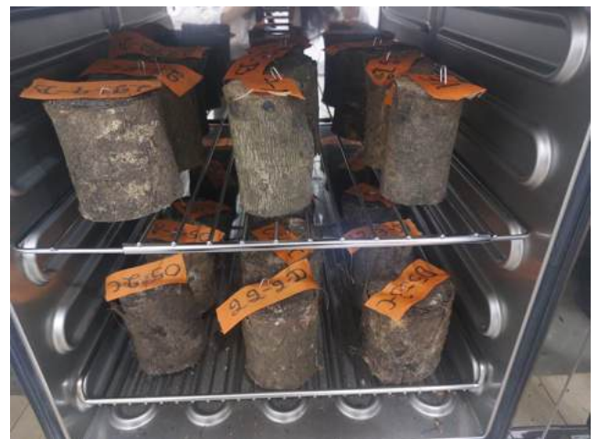
Figure 53: WP5 experiment: cut sections of wood dried at 80 °C until the mass remains constant
